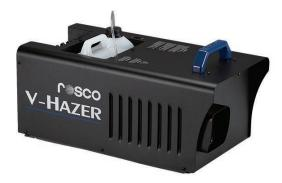
Fan and pump speed are synchronized to a single potentiometer to create an optimal haze effect when controlled via the detachable remote. Independent control of fan speed and pump volume is available via two channels of DMX, which allows the user to dial in their perfect balance of fast haze time and even distribution. To maintain the quietest performance environment, the V-Hazer was designed with a silent mode; after 30 seconds of inactivity, the fan switches off for truly silent operation.
