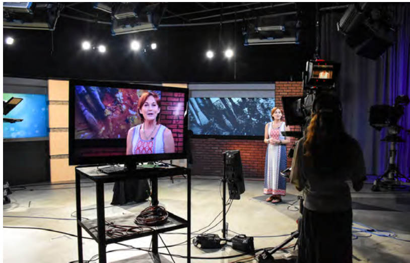
Several pairs of Rosco Braq Cube WNC LED fixtures backlight the KNPB ARTEFFECTS set
