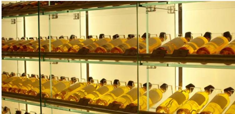
The lighting designers at Speirs + Major used light to create the store's upscale identity and to develop its glowing character. They knew going in that, in order to facilitate the optimum temperature for its products, the store would be lit 100% with cool-running LEDs.
