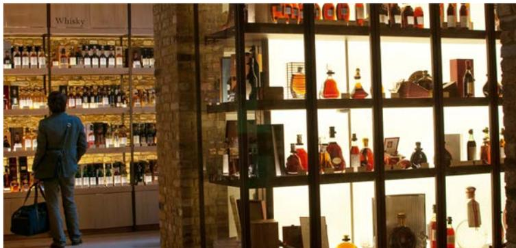
One of the major design goals of the project was to imperceptibly integrate the lighting into the architecture – maintaining the customer’s focus on the merchandise, not the light fixtures. With three levels of premium product to illuminate, the design team turned to Rosco’s Custom LitePad and its slim (8mm), easy-to-install form-factor to backlight the bottles.
