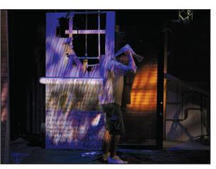
Rosco's Infinity was affixed to two overlapping spotlights to generate this realistic rain effect. Both spotlights included a Water 1 gobo (No.77833) in their gates. The Infinity in one unit was disk 30019, in the other disk 30011.
