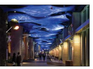
The designers at Focus Lighting found a brilliant solution to projecting rippling water on the ceiling of The Pier in Caesars Atlantic City. X-Effects Projectors, mounted down the length of the mall shopping area, gave them the effect they wanted.
