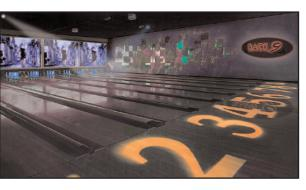
The designers at Simply By Others used gobos to mark the lane numbers at this 300 San Jose AMF Bowling Center. This clever method to draw attention to an area is flexible and cost effective. A rippling water effect is added to the side walls with the X24 X-Effects projector.
